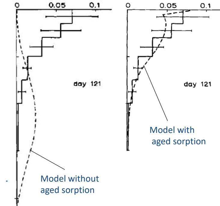
Simulated measured cyanazine depth profiles with and without aged sorption model (Boesten 1989)
